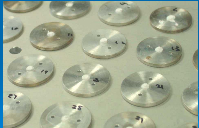
X-ray Filter Stage and Holder (patented)
